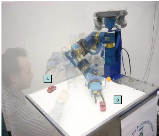
Fig. 7. The robot arm tracks a target which is displaced by the human operator during arm movement
