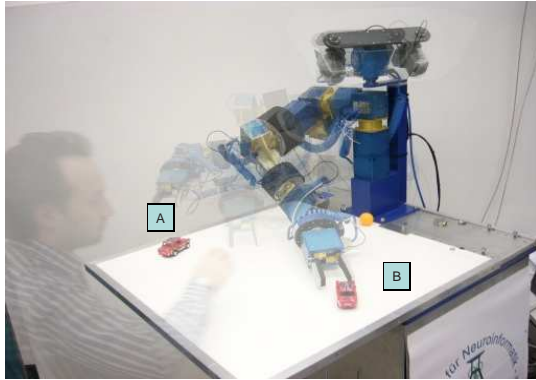
Fig. 7. The robot arm tracks a target which is displaced by the human operator during arm movement
